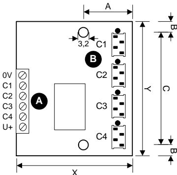
**A** Output supply voltage and I/O terminals C1 – C4
